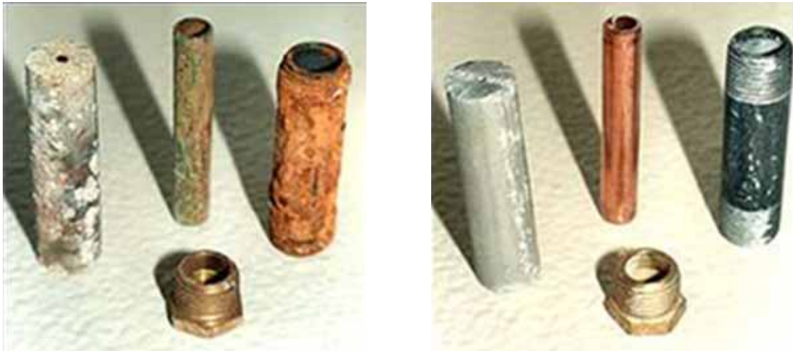
Untreated Water Circuit
