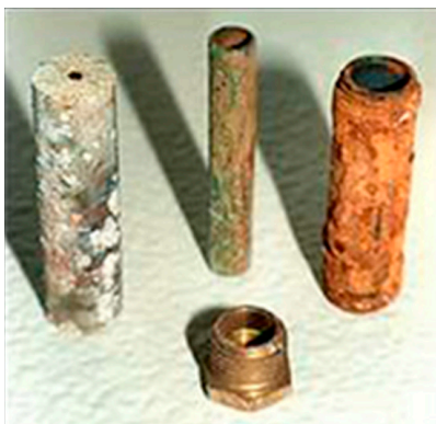
Untreated Water Circuit
