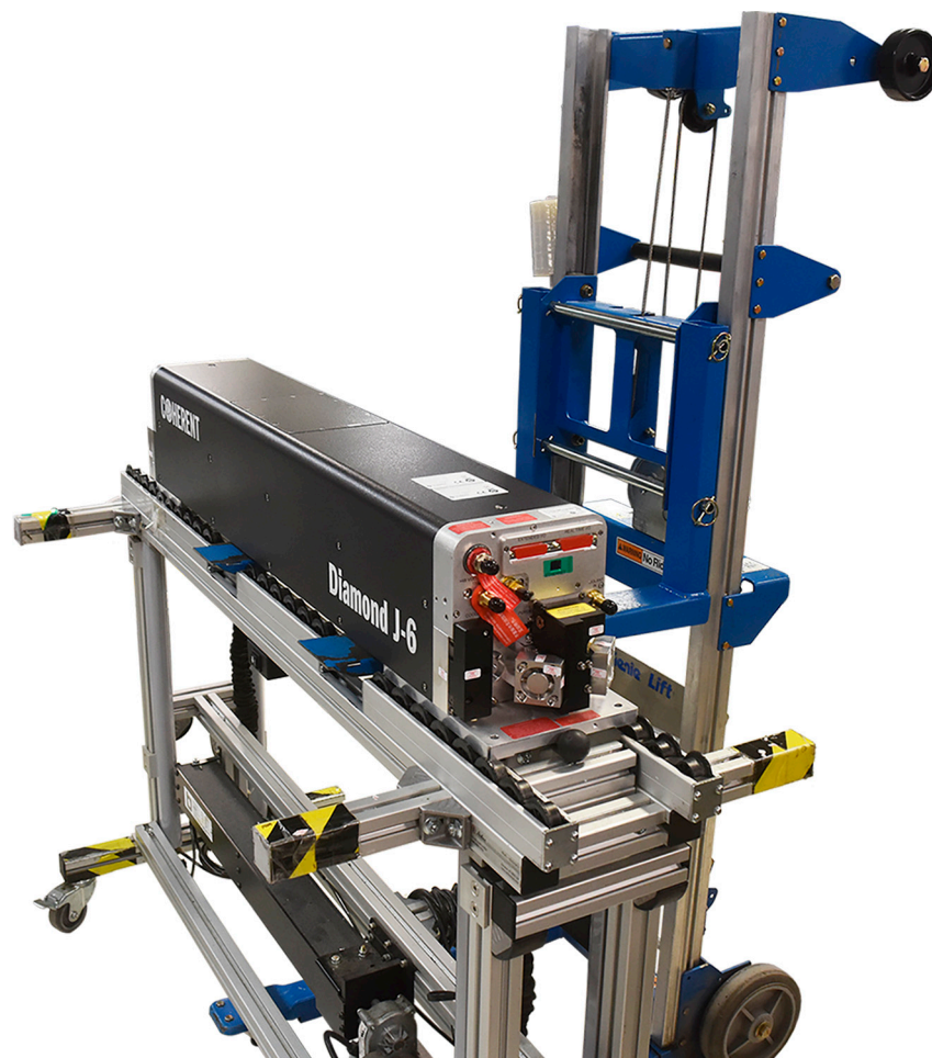
Figure 4-9. Lifting the Laser (Continued)
