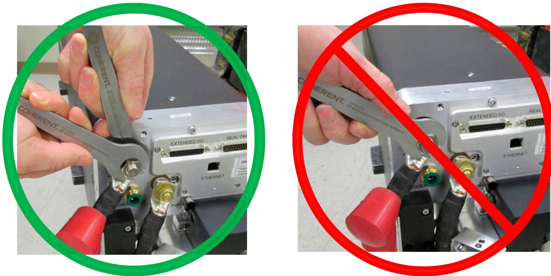
Figure 4-17. +48 VDC Location and Using Two Wrenches
