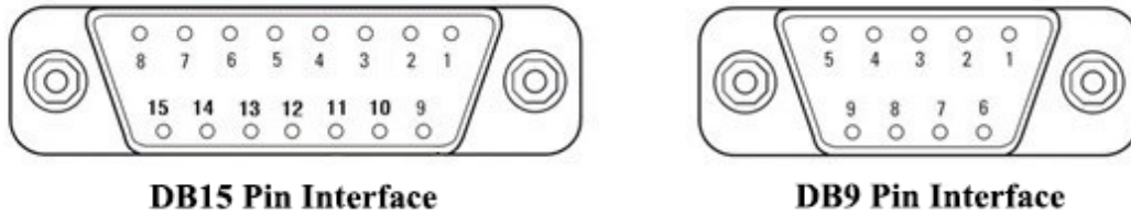
Figure 9 Pin Connection Description
