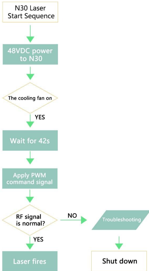
N30 (air-cooled) operational flowchart
