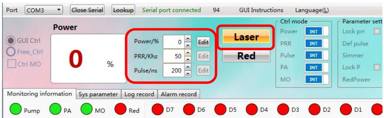
**Figure 21 Setting parameters and emitting**
