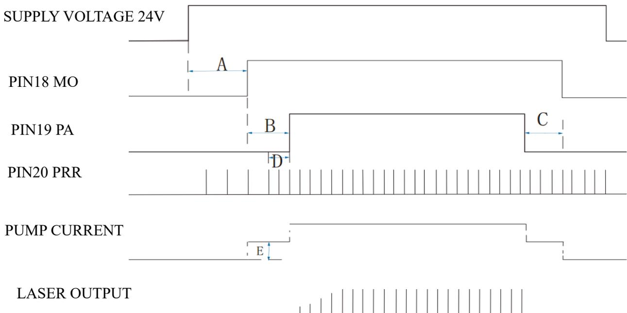
**Figure 15 DB25 Controlling Time Series Diagram**
