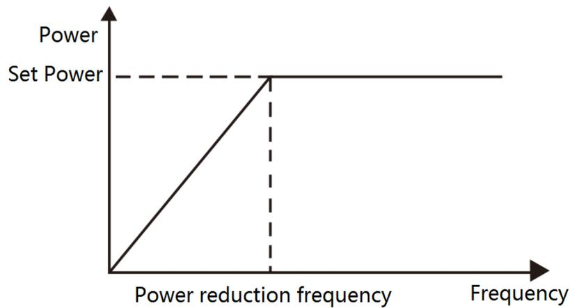
**Figure 4 Power reduction frequency & Output power relationship charts**
