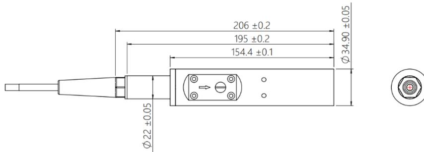
**Figure 8** YDFLP-E-20-LP-S Standard isolated output head dimensions (Unit: mm)
