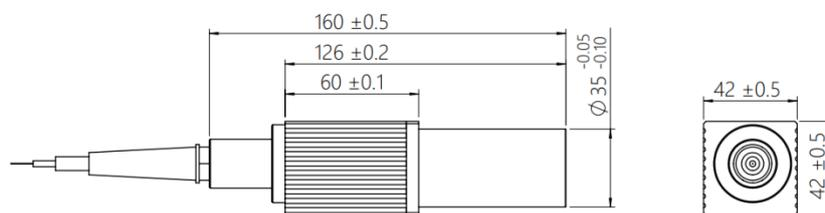
**Figure 9** YDFLP-E-30-LP-S Standard isolated output head dimensions (Unit: mm)
