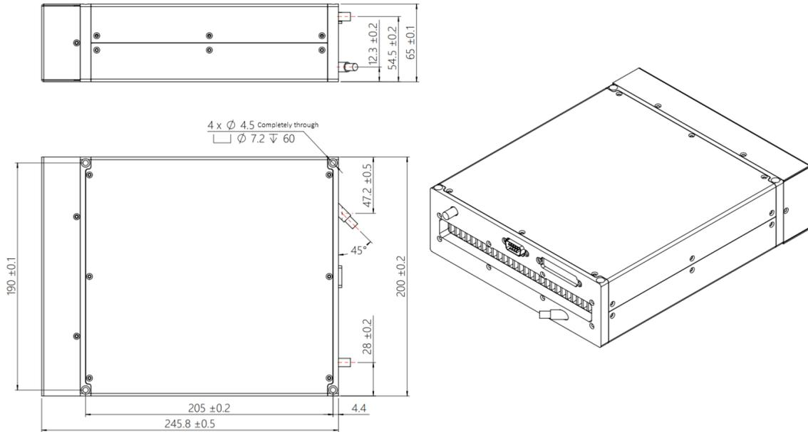
**Figure 7** YDFLP-E-20&30-LP-S Laser module dimensions (Unit: mm)
