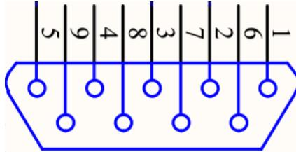
**Figure 13 RS232 connector DB9**
