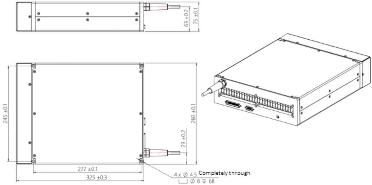
**Figure 10** YDFLP-E-50-LP-L Dimensions of fiber laser module (Unit: mm)
