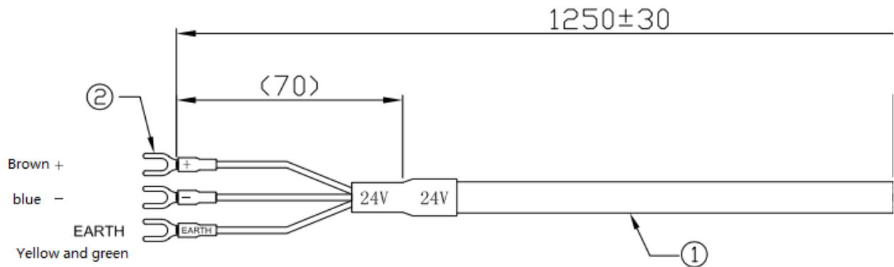
**Figure 12** Diagram of the power supply cable
