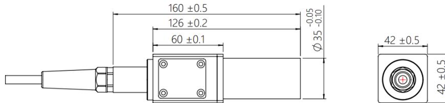
**Figure 11** YDFLP-E-50-LP-L Dimensions of fiber laser module (Unit: mm)
