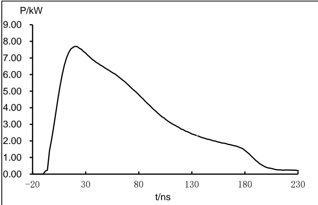
Figure 5 YDFLP-E-20&30-LP-S Output waveform graph
