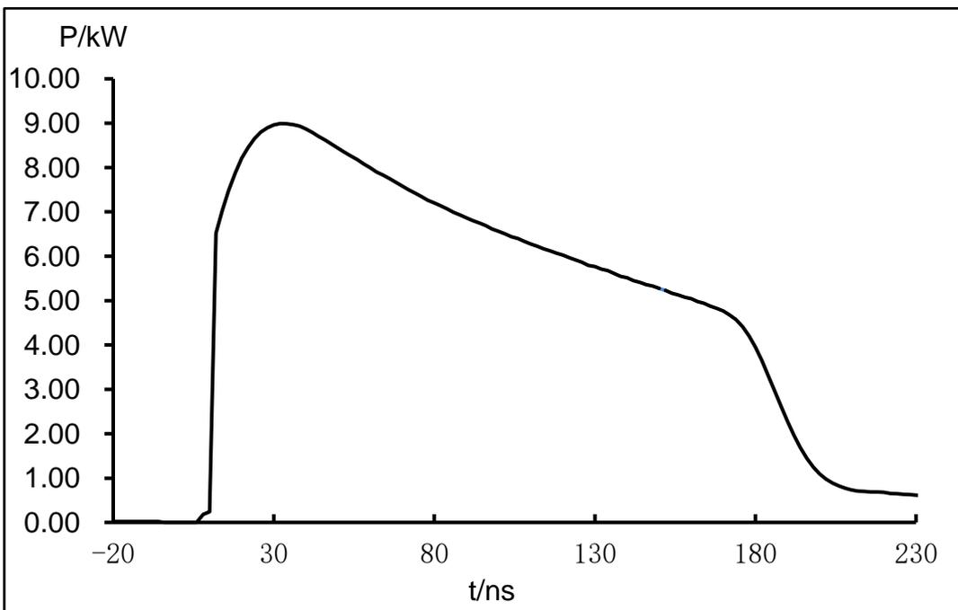
Figure 6 YDFLP-E-50-LP-L Output waveform graph
