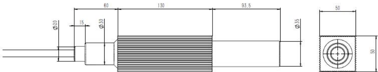
Figure 2 Dimension drawing of output isolator (Unit: mm).
