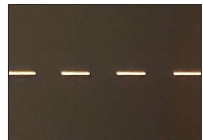
In this example the thin film was cut using a Synrad vi30+, yielding clean, consistent cuts.
