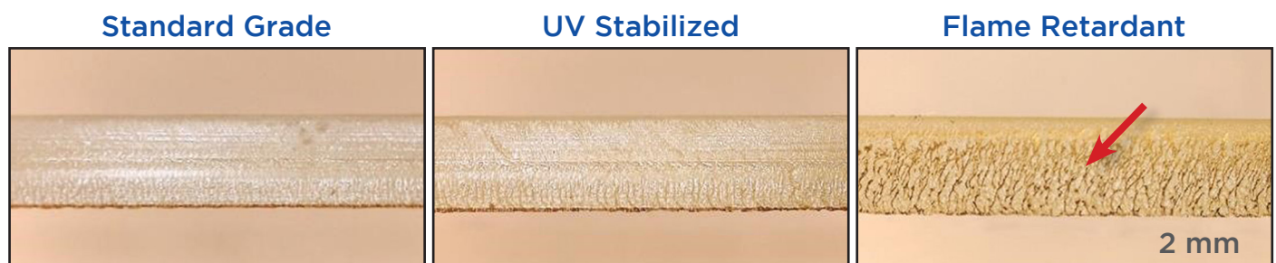
Three different types of PC cut with the same processing parameters
